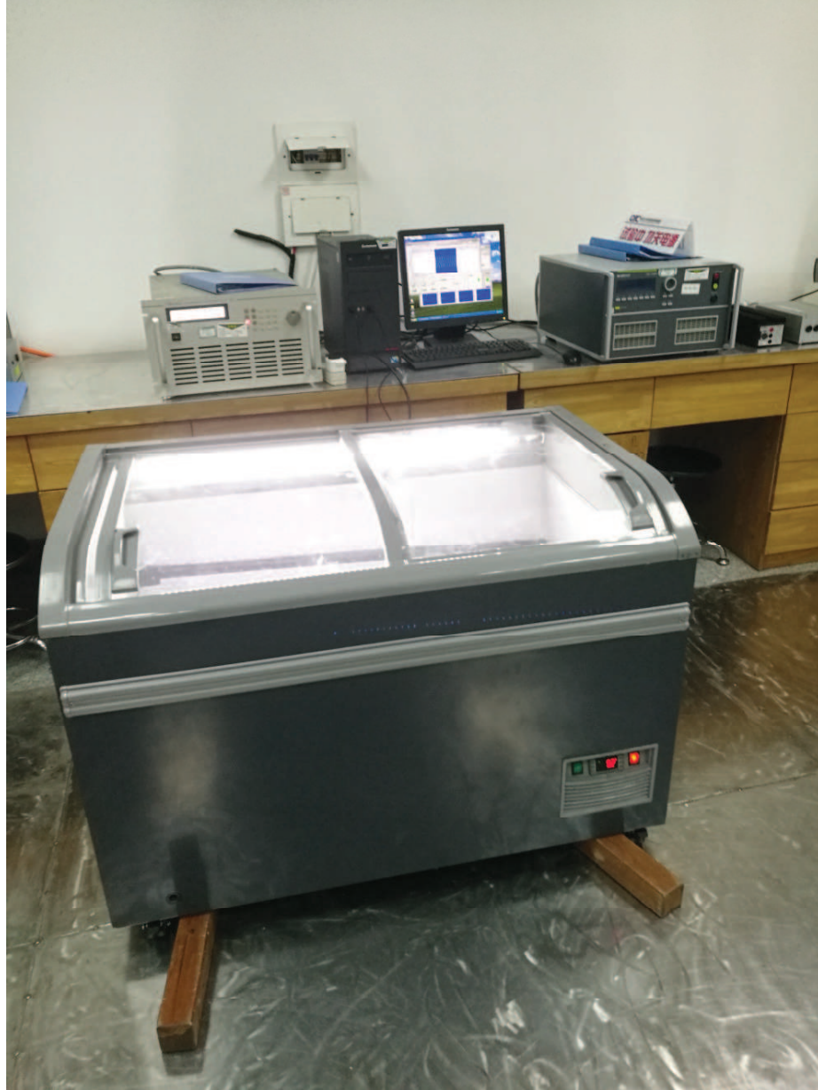
Photograph 6: Set-up for Voltage Dips
