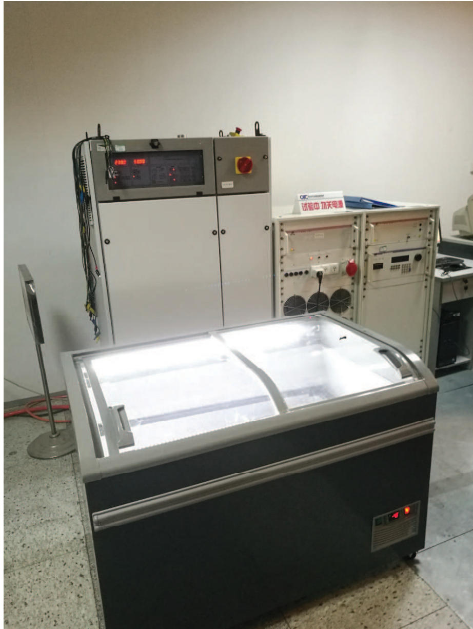
Photograph 1: Set-up for Harmonics, Voltage Fluctuations and Flicker
